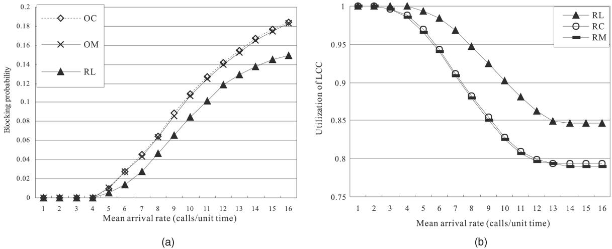
Fig. 17.  $SF = 64$ ,  $\alpha = 5$ : (a) blocking probability at different traffic loads and (b) utilization of linear-code chains.
