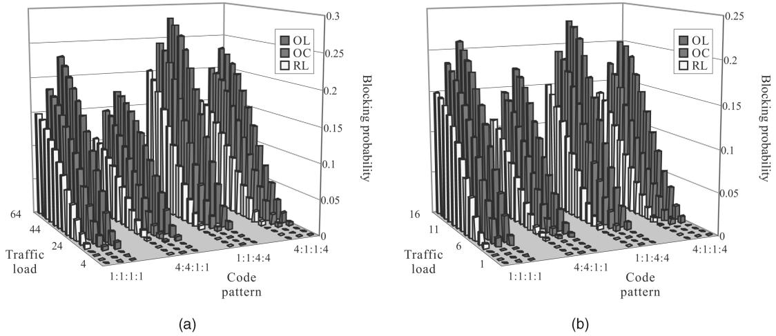
Fig. 21. Effects of different call patterns on code blocking probabilities: (a)  $SF = 256, \alpha = 5$  and (b)  $SF = 64, \alpha = 5$ .
