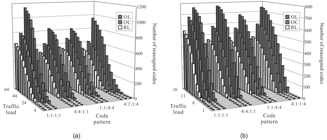
Fig. 22. Effect of different call patterns on code reassignment costs: (a)  $SF = 256, \alpha = 5$  and (b)  $SF = 64, \alpha = 5$ .
