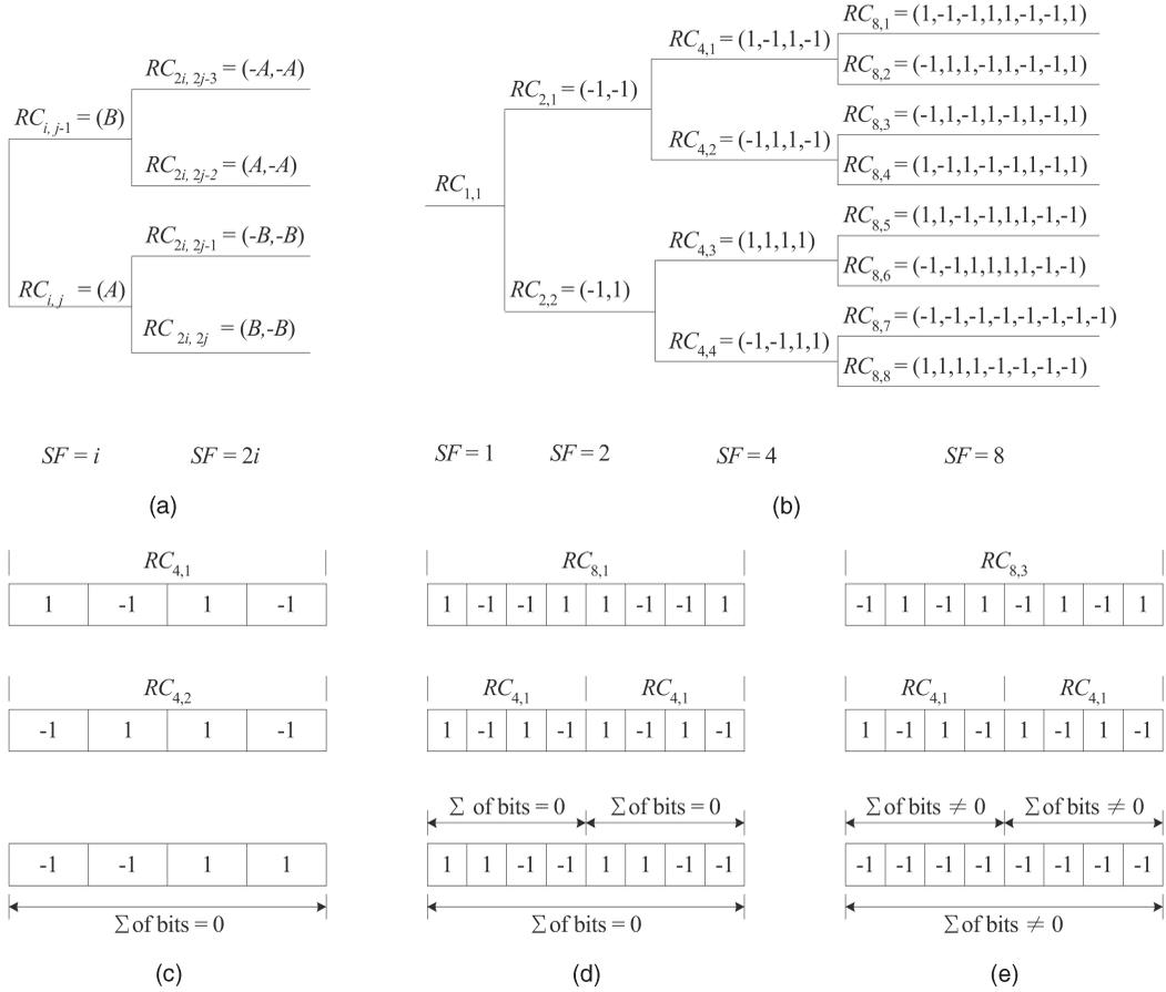
Fig. 2. A rotated OVFSF (ROVSF) code-tree.
