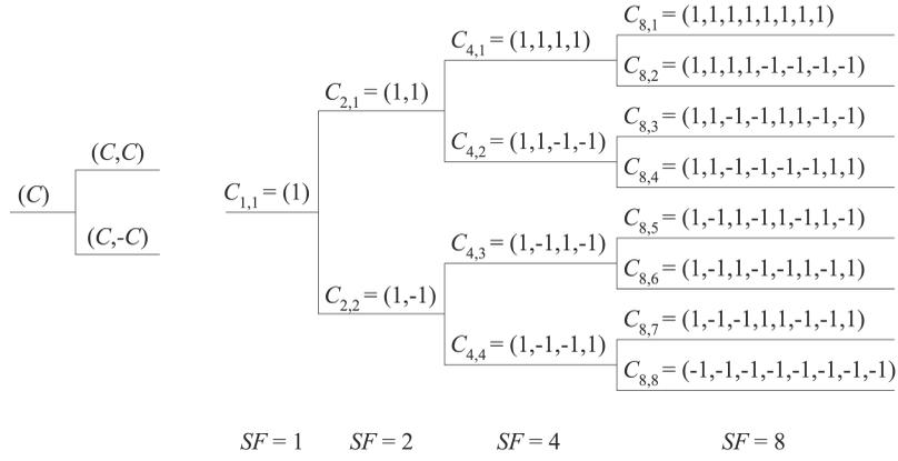
Fig. 1. An orthogonal variable spreading factor (OVSF) code-tree.
