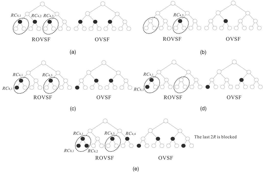
Fig. 12. Example of code placement using our scheme and the OVSF+crowded-first scheme. (a)  $2R$ ,  $2R$ , and  $2R$  are coming. (b) The first and third  $2R$ s are released. (c)  $1R$  and  $2R$  are coming. (d) The second  $2R$  is released. (e)  $1R$ ,  $2R$ , and  $2R$  are coming.
