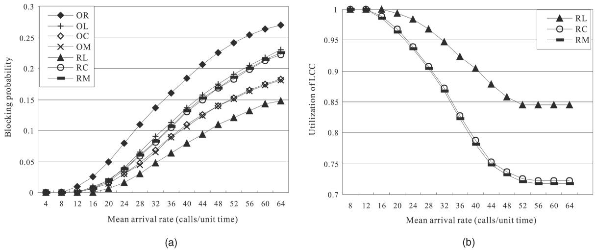
Fig. 16.  $SF = 256$ ,  $\alpha = 5$ : (a) blocking probability at different traffic loads and (b) utilization of linear-code chains.
