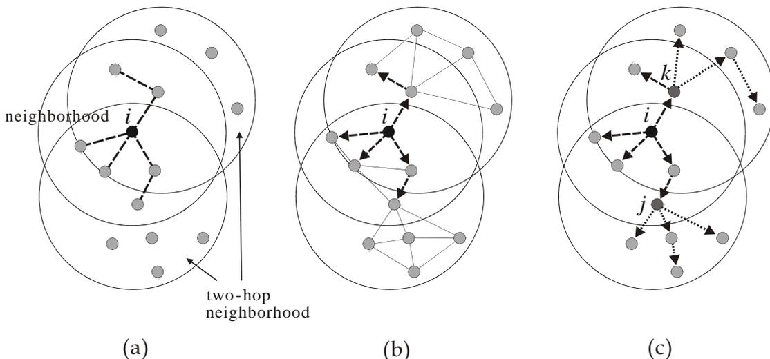
**Fig. 6:** (a) local BIP tree for node  $i$ , (b) Dist-BIP-A tree, and (c) Dist-BIP-G tree
