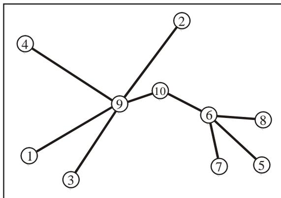
**Fig. 2:** Broadcast tree using BIP
