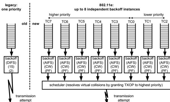
Fig. 5: Virtual backoff of eight traffic categories: (1) left one: legacy DCF, close to EDCF with  $AIFS=34\mu s$ ,  $CWmin=15$ ,  $PF=2$ ; (2) right one: EDCF with  $AIFS[TC] \geq 34\mu s$ ,  $CWmin[TC]=0-255$ ,  $PF[TC]=1-16$ .
