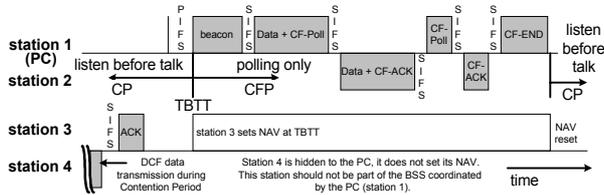
Fig. 2: Example for the PCF operation. Station 1 is the PC polling station 2. Station 3 detects the beacon frame and sets the NAV for the whole CFP. Station 4 is hidden to station 1 and does not detect the beacon frame; it continues to operate in DCF.
