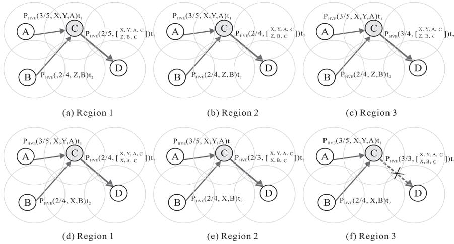
Fig. 5. Merging operations for cluster heads.
