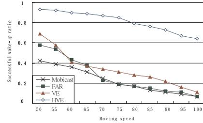
Fig. 9. The successfully woken-up ratio v.s. moving speed.
