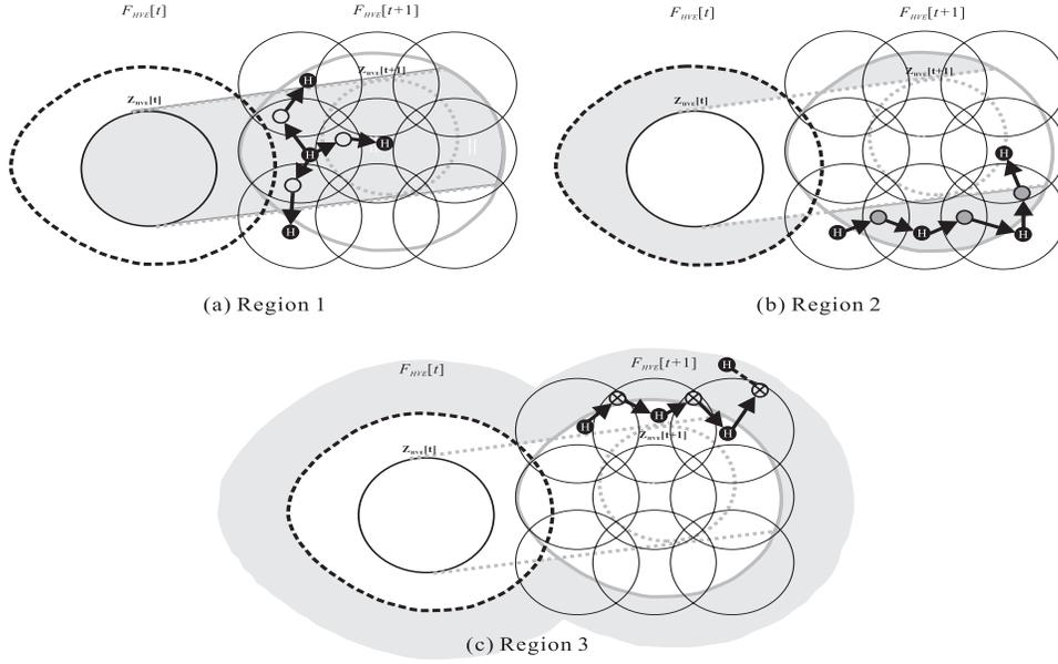
Fig. 4. Forwarding rules for relay nodes in three different regions.
