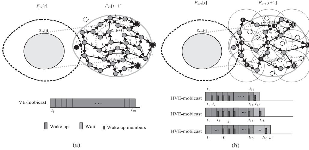
Fig. 1. Waking up process with the VE-mobicast and HVE-mobicast protocol.
