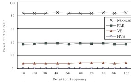
Fig. 6. The packet overhead ratio vs. the rotation frequency.
