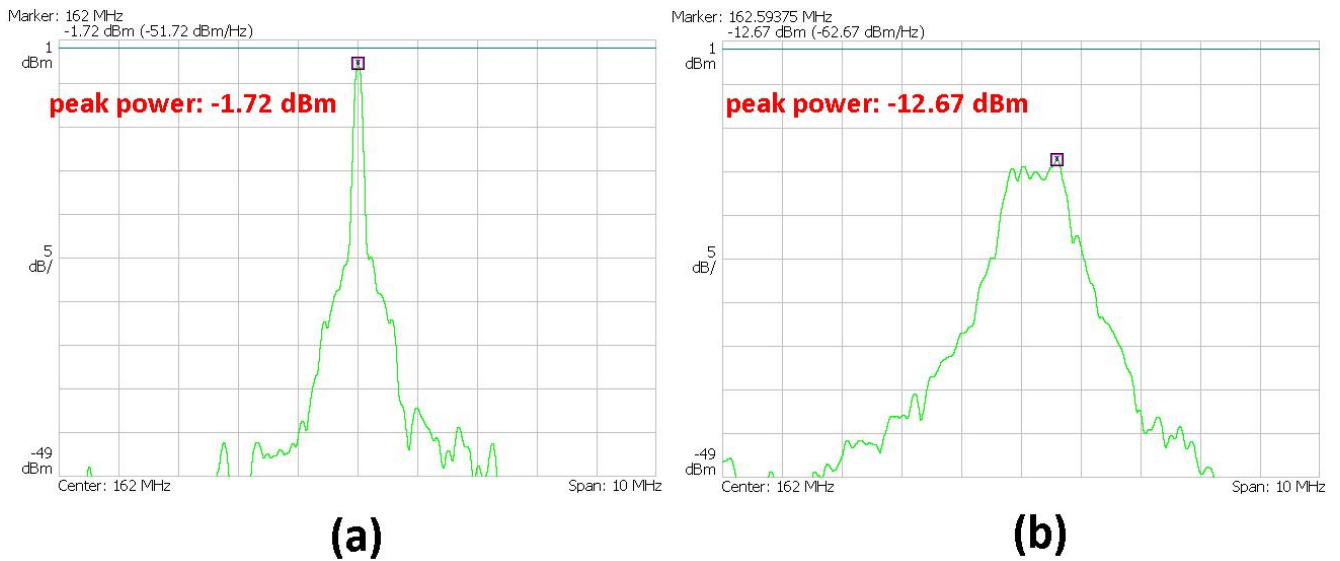
Fig. 5.8: Power spectral density at 162MHz (a) spread-spectrum off state (b) spread-spectrum clock with 0.5% spreading ratio.
