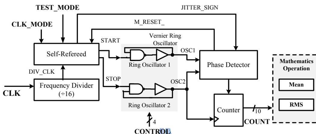
Fig. 2-14 The structure of proposed built-in jitter measurement (BIJM) [46]
