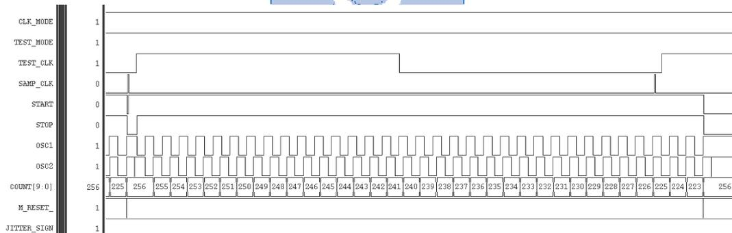
Fig. 4-6 The timing diagram of the proposed BIJM circuit in normal mode
