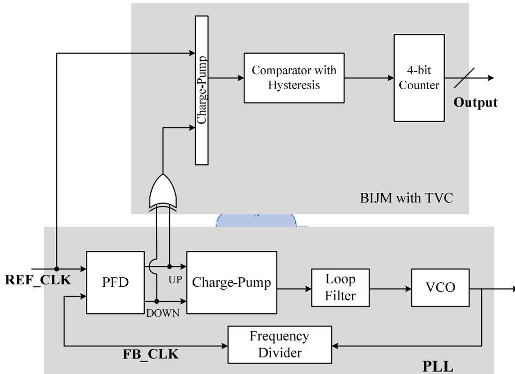
Fig. 2-10 The structure of the BIJM circuit with TVC technique
