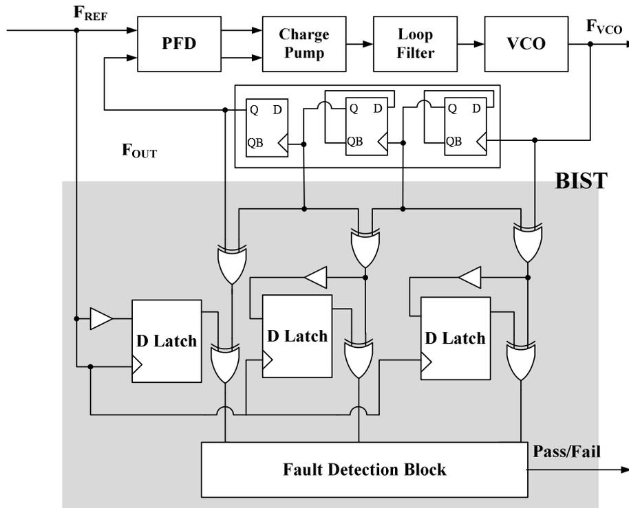
Fig. 3-2 The BIST structure with directly invasive testing [34]
