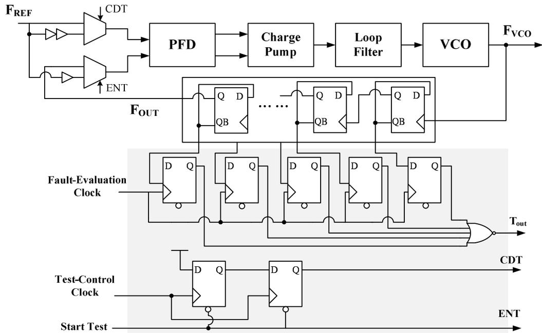
Fig. 3-3 The BIST structure with indirectly invasive testing [35]
