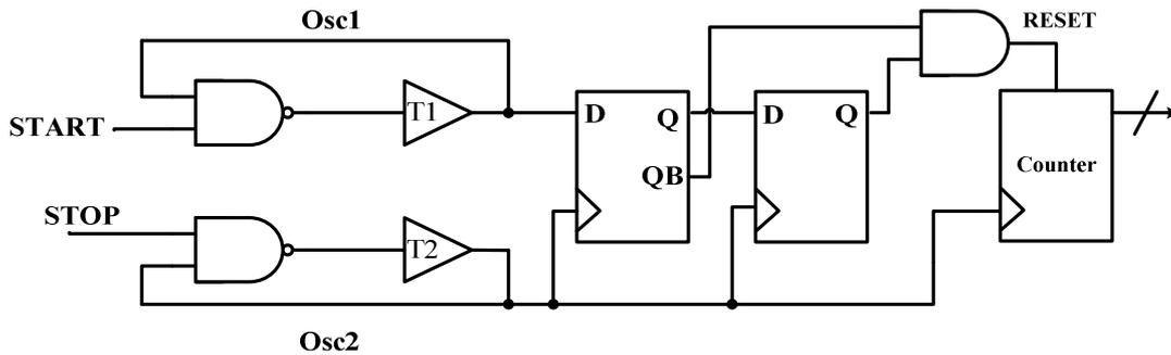
Fig. 2-8 The structure of vernier ring oscillator [16]
