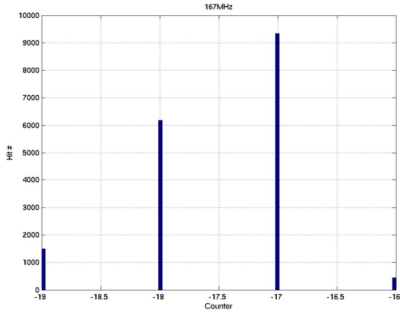
Fig. 4-8 The jitter histogram measured by the proposed BIJM chip
