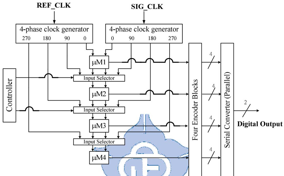
Fig. 2-9 The structure of the BIJM with interpolated technique
