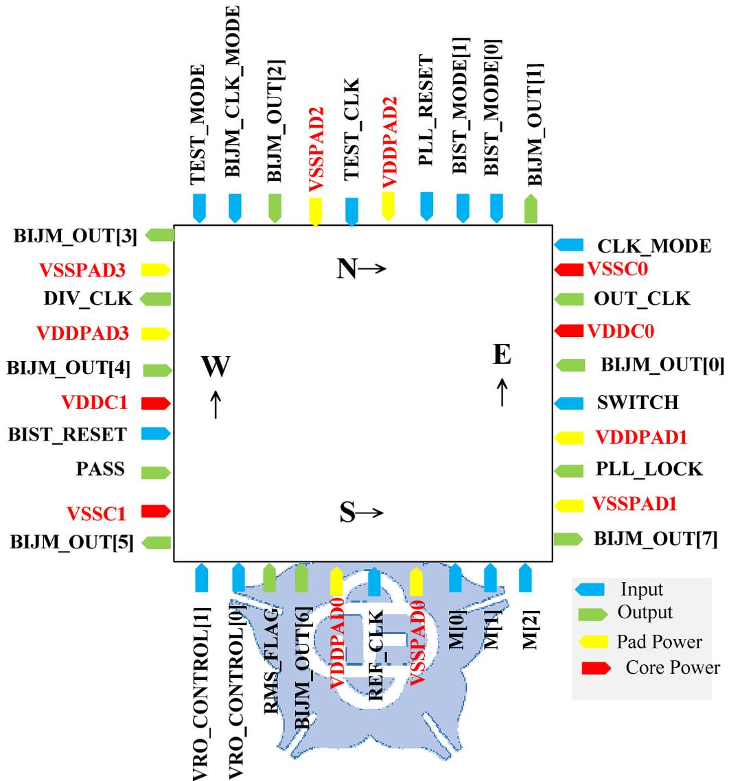
Fig. 4-11 The proposed BIJM chip floorplanning and I/O planning
