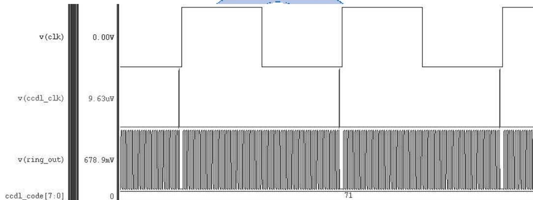
Fig. 4-4 The simulation result of the CCDL circuit.
