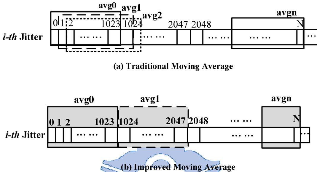
Fig. 2-25 The concept of moving average-(a) conventional moving average, (b) improved moving average
