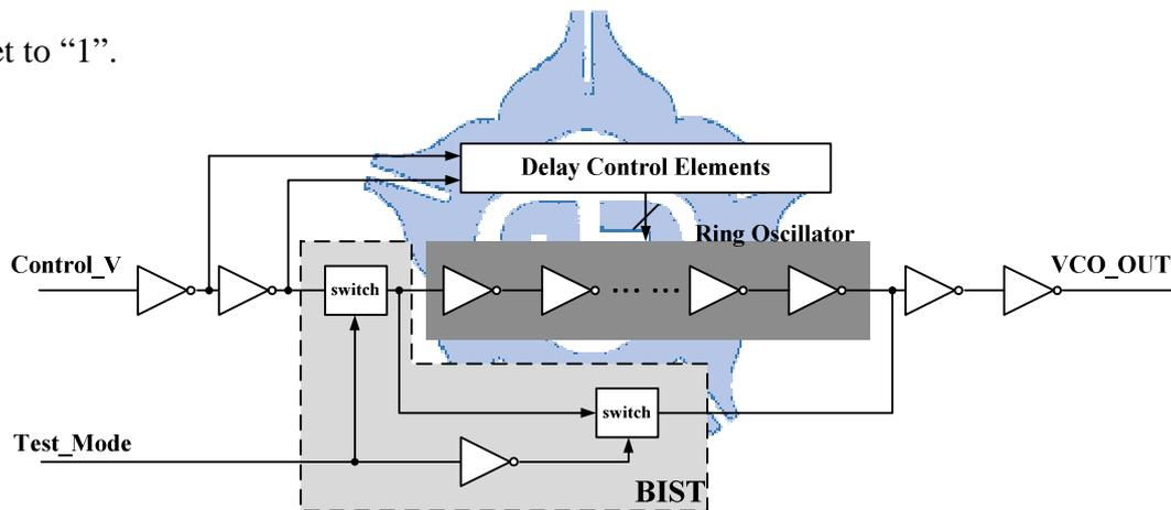
Fig. 3-4 The BIST structure in open loop testing [41]
