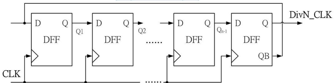
Fig. 2-16 The structure of a Johnson counter
