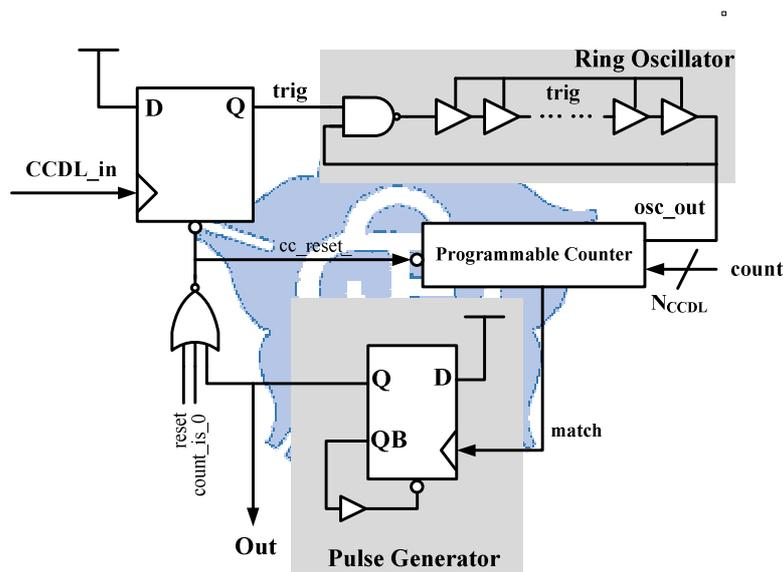
Fig. 2-20 The structure of cycle-controlled delay line (CCDL) [43]
