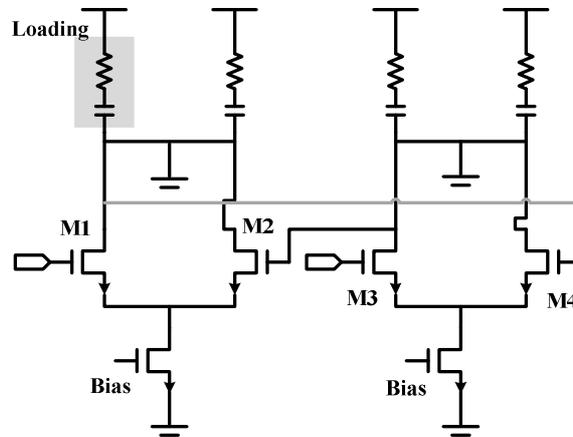
Fig. 2-5 The schematic of analog timing amplifier [45]
