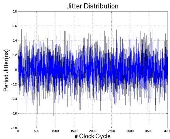
Fig. 2-24 The jitter distribution with radon variables
