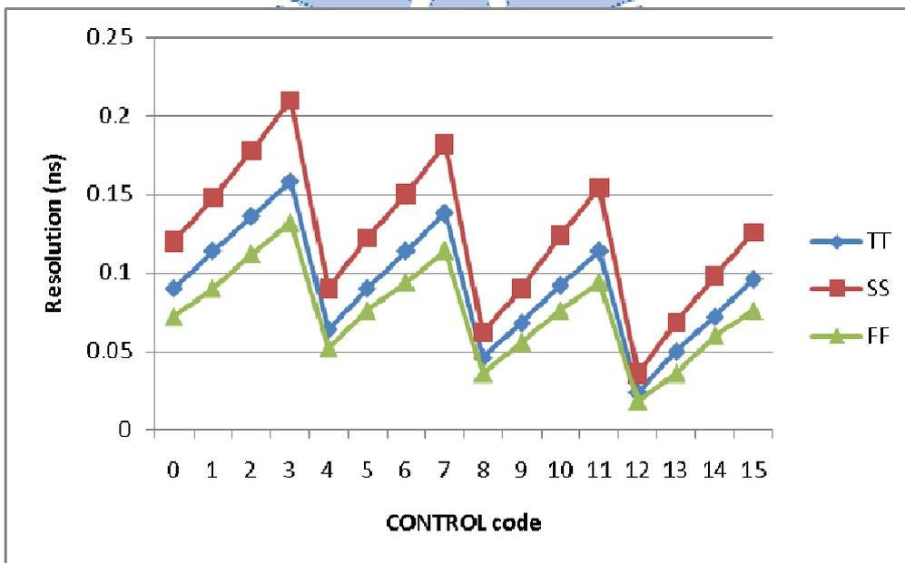
Fig. 4-5 The comparison of the VRO resolution in PVT
