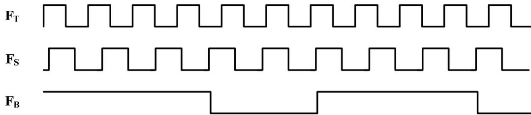
Fig. 2-12 The timing diagram of the BIJM circuit with sampling technique
