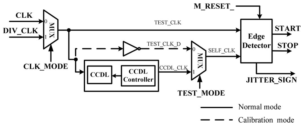
Fig. 2-17 The proposed self-referred circuit
