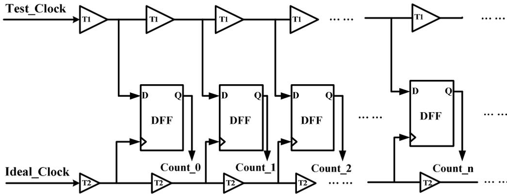
Fig. 2-7 The simple structure of vernier delay line (VDL)
