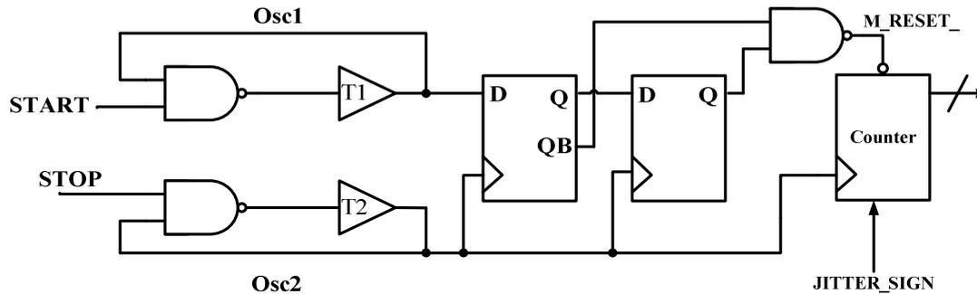
Fig. 2-22 The structure of vernier ring oscillator (VRO) [18]
