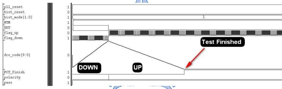
Fig. 4-13 The simulation result of BIST for PFD testing
