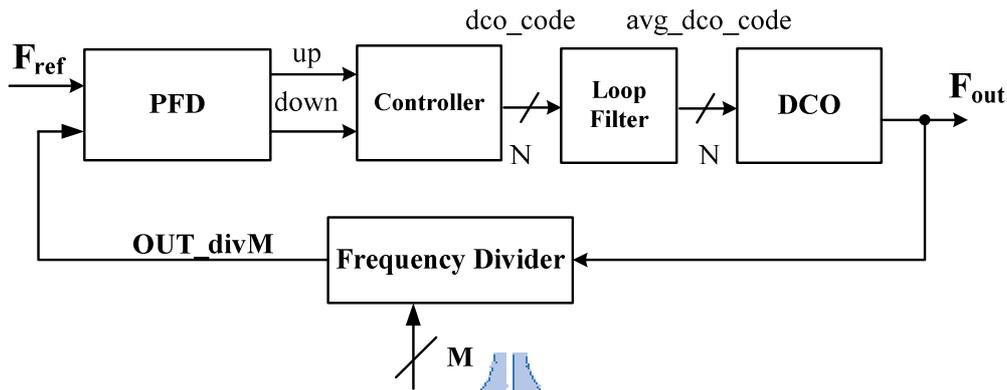
Fig. 1-2 The architecture of all-digital phase-locked loop (ADPLL)
