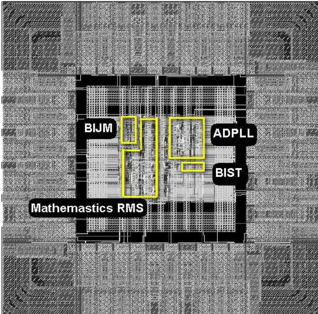
Fig. 4-12 The layout of the proposed BIST circuit
