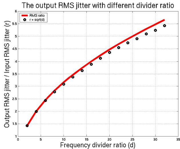
Fig. 2-15 The relationship of the input and output RMS jitter
