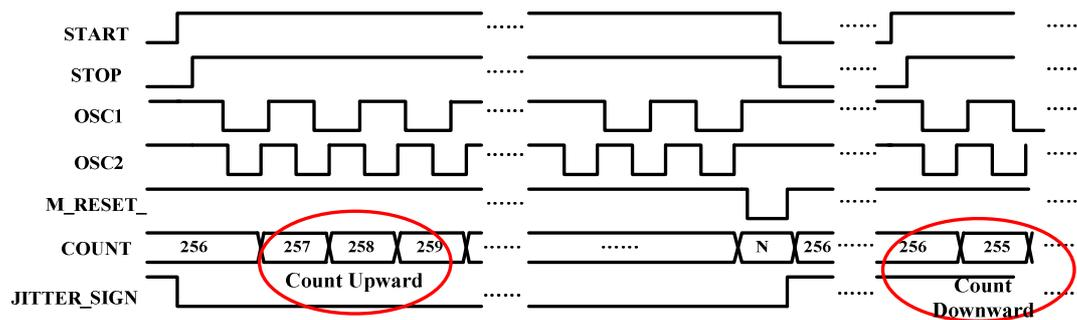
Fig. 2-23 The timing diagram of the VRO and the PD in BIJM circuit.
