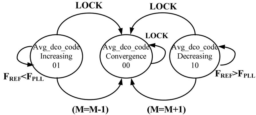
Fig. 3-9 The state machine of PLL locking in BIST for divider testing
