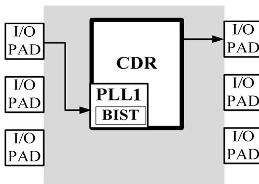
Fig. 3-10 The application environment of single PLL
