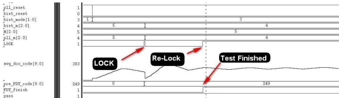
Fig. 4-14 The simulation result of BIST for frequency divider testing
