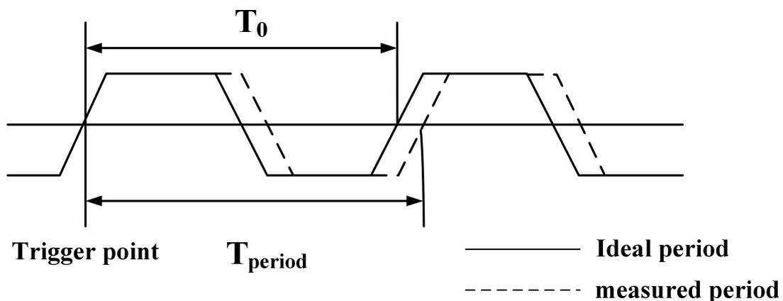
Fig. 2-2 The definition of period jitter ( $J_{\text{period}}$ )
