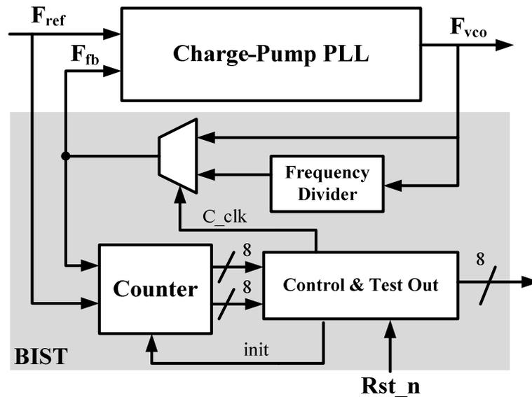
Fig. 3-1 The structure of BIST in non-invasive testing [33]
