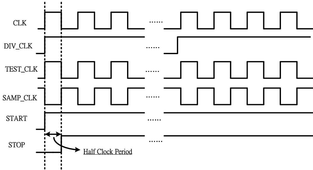
Fig. 2-18 The timing diagram of the calibration mode
