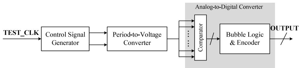
Fig. 2-11 The structure of the BIJM circuit with ADC technique
