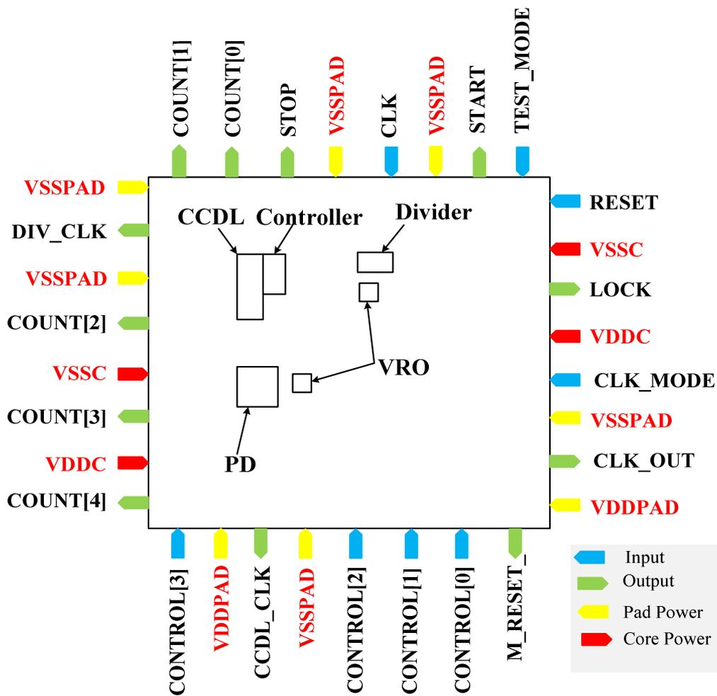
Fig. 4-2 The proposed BIJM chip floorplanning and I/O planning
