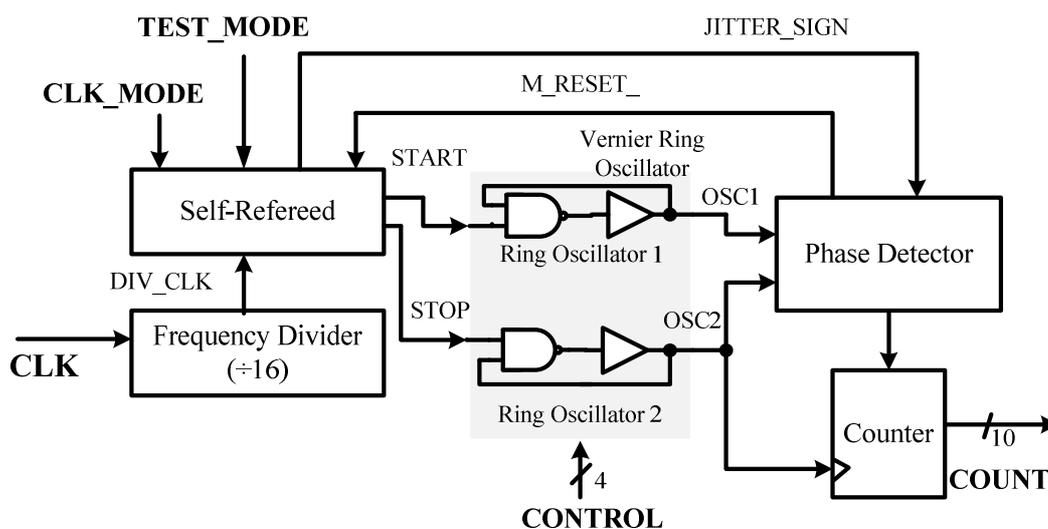
Fig. 4-1 The architecture of the proposed BIJM circuit
