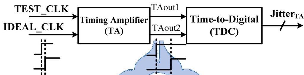
Fig. 1-3 The concept of built-in jitter measurement with timing amplifier
