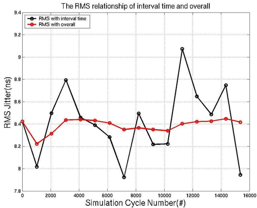
Fig. 2-26 The relationship of the interval time RMS and the overall time RMS
