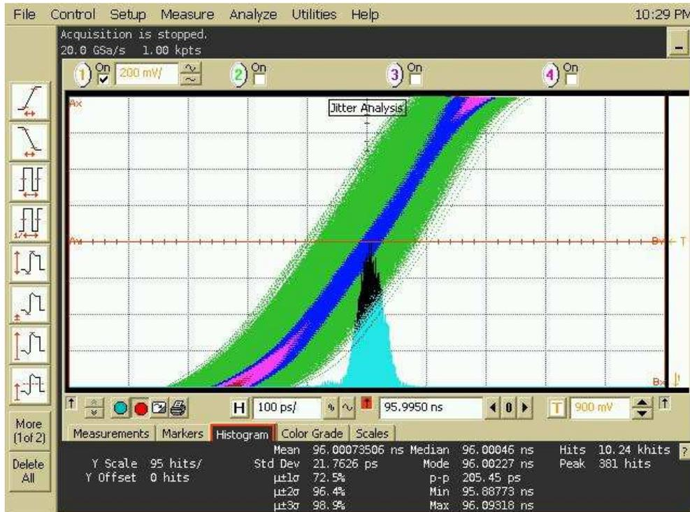
Fig. 4-7 The jitter histogram in oscilloscope
