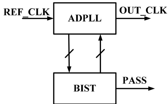
Fig. 4-10 The simple architecture of the proposed BIST circuit with PLL
