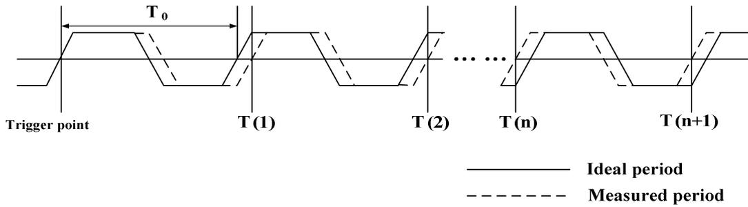
Fig. 2-4 The N-cycle definition ( $J_{long}$ )
