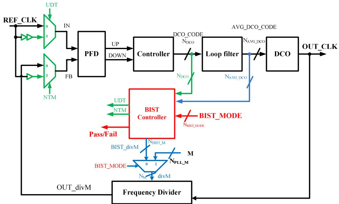
Fig. 3-6 The architecture of the BIST sub-circuit.
