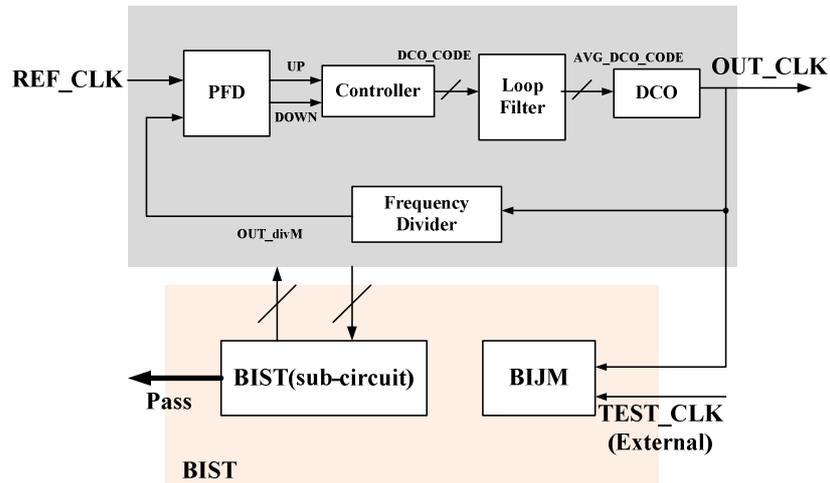
Fig. 3-5 The proposed BIST for PLL structure
