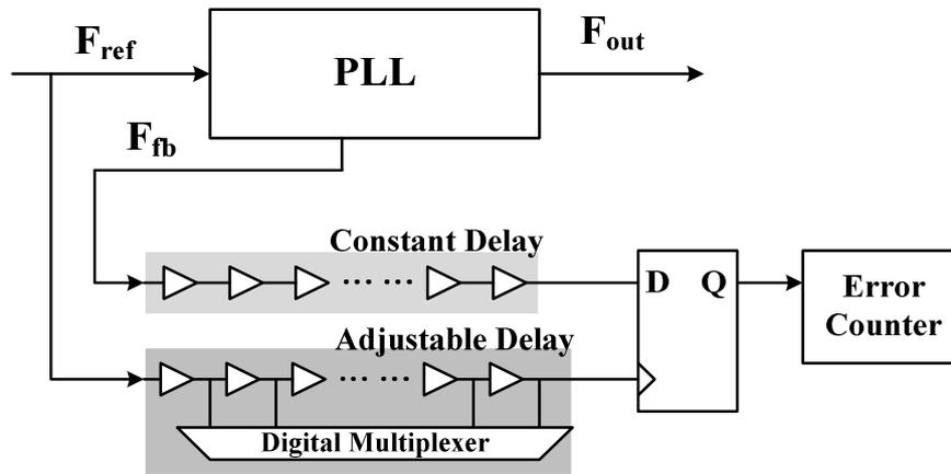
Fig. 2-6 The delay line for jitter measurement [7]
