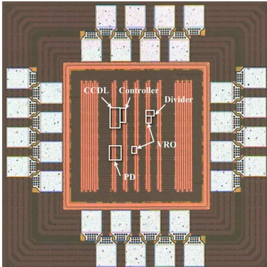
Fig. 4-3 The microphotograph of proposed BIJM circuit
