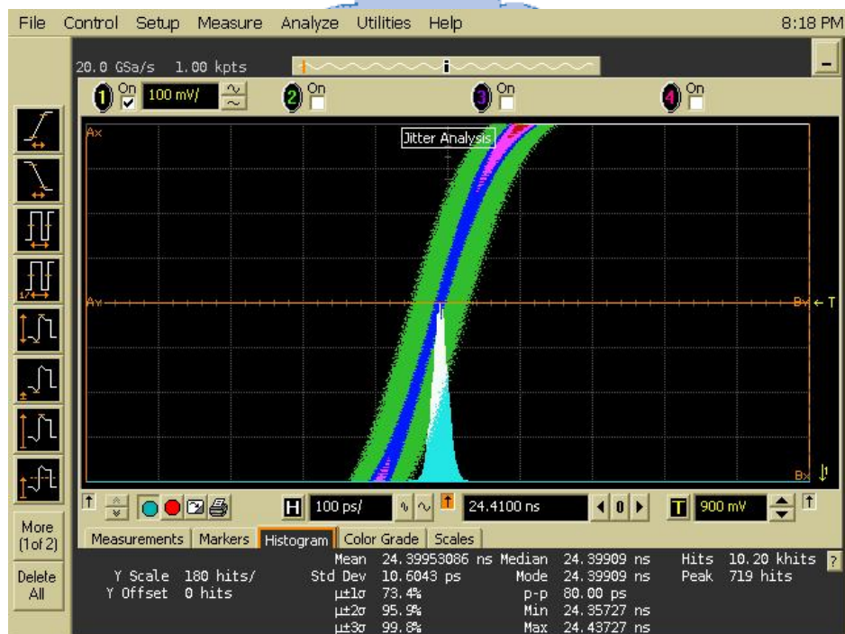
(d) Jitter histogram of on-chip clock generator output clock 325MHz and output is divided by 8
