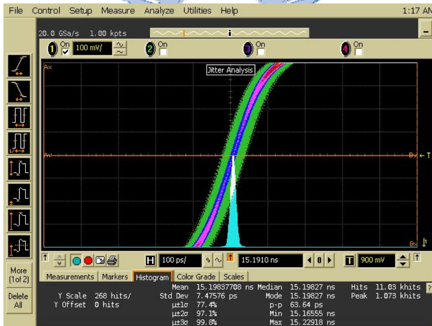
(b) Jitter histogram of the on-chip clock generator clock at 526MHz and output is divided by 8
