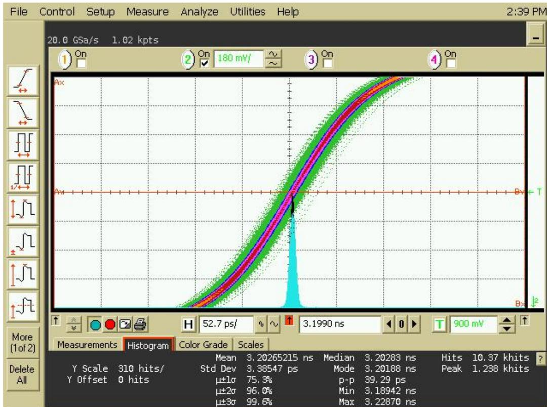
Fig. 4.11 Measured long-term jitter histogram (at 1.2 GHz).
