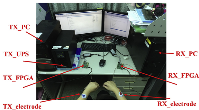
Fig. 14. The measurement environment of the proposed BCC transceiver.
