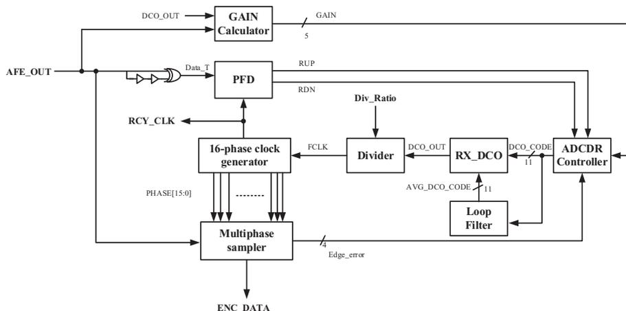
Fig. 7. The block diagram of the proposed ADCDR circuit.
