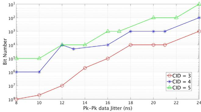
Fig. 13. Error-Free simulation result at 20 Mbps with different CID.
