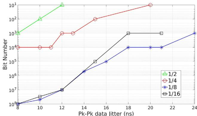
Fig. 15. Error-Free simulation result at 20 Mbps with different gain ratio.
