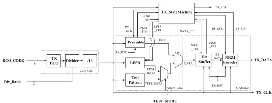
Fig. 2. Architecture of the proposed WBS BCC transmitter.
