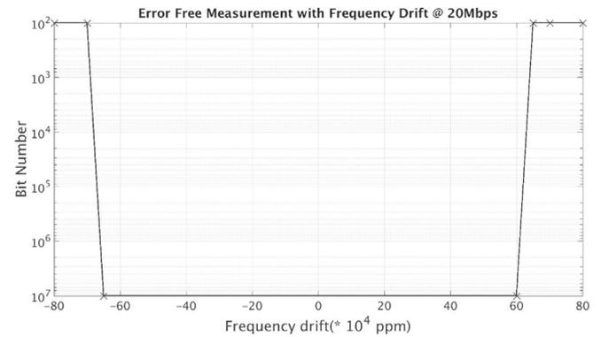
Fig. 17. Error-Free measurement with different frequency drift at 20 Mbps
