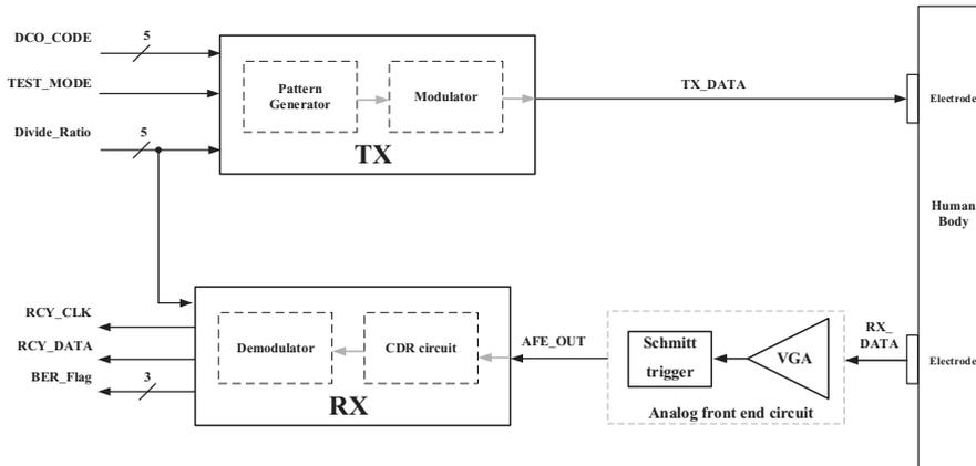
Fig. 1. Architecture of the proposed WBS BCC transceiver.
