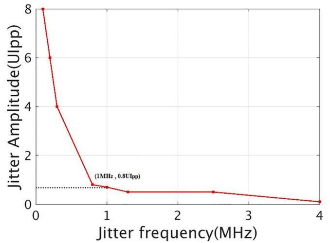
Fig. 16. Sinusoidal jitter tolerance performance.
