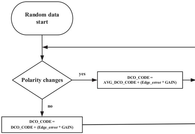
Fig. 9. Compensation flow with random data input.
