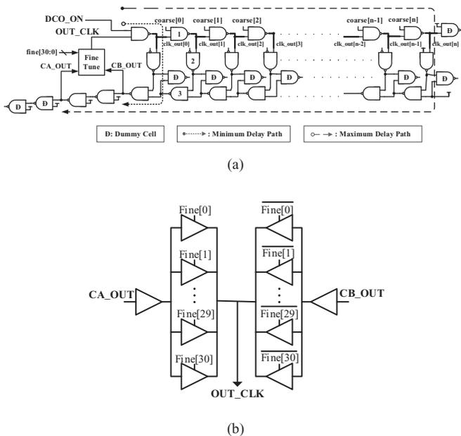
Fig. 10. (a) The proposed DCO (b) The fine-tuning circuit of the proposed DCO.
