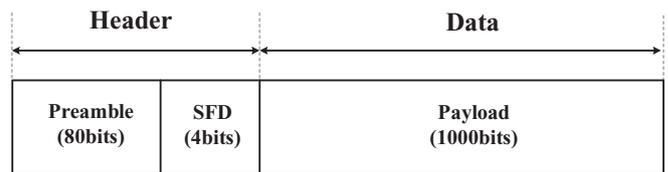
Fig. 3. The packet format of the WBS BCC transceiver.
