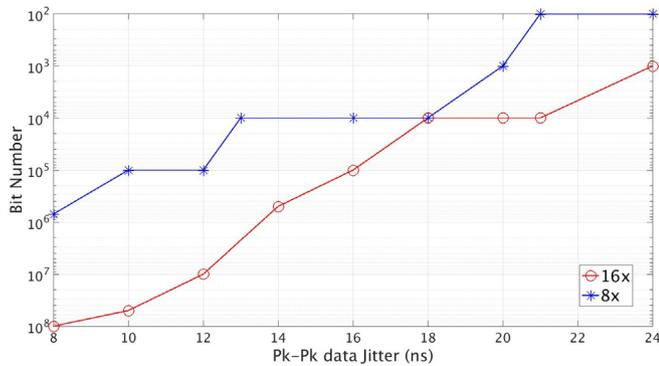
Fig. 14. Error-Free simulation result at 20 Mbps with different oversampling rate.
