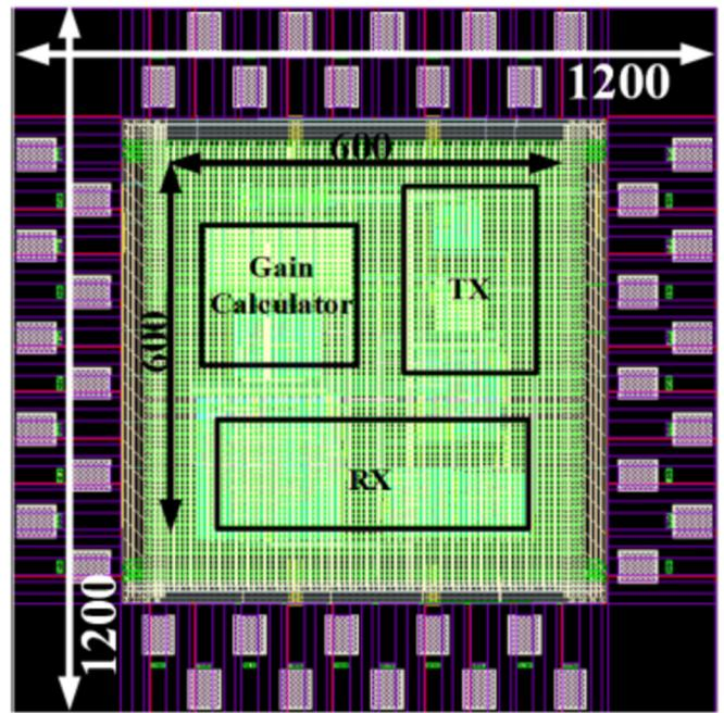
Fig. 11. Layout of the proposed WBS BCC transceiver.
