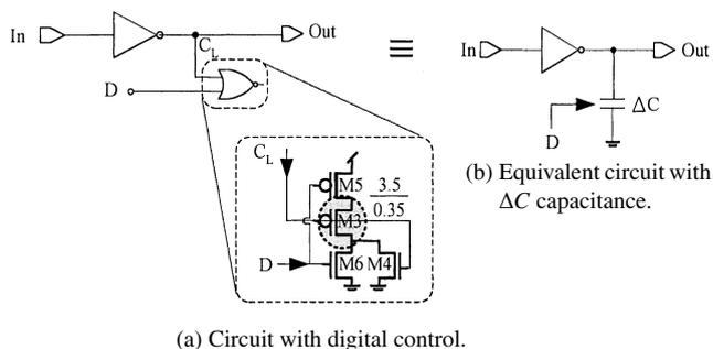
Fig. 2 Proposed digitally-controlled varactor (DCV).
