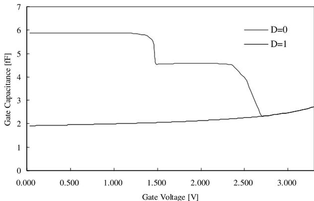
Fig. 3 Variations of two-input NOR gate’s capacitance corresponding to  $D = 0$  and  $D = 1$ .
