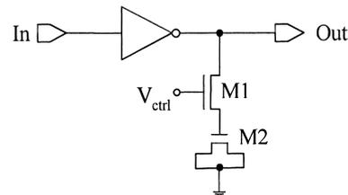
Fig. 1 Conventional delay element with shunt capacitor.
