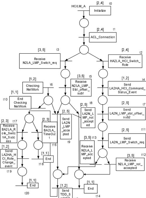
**Figure 3. TCCPN model of HC/LM A in Bluetooth M/S switch**
