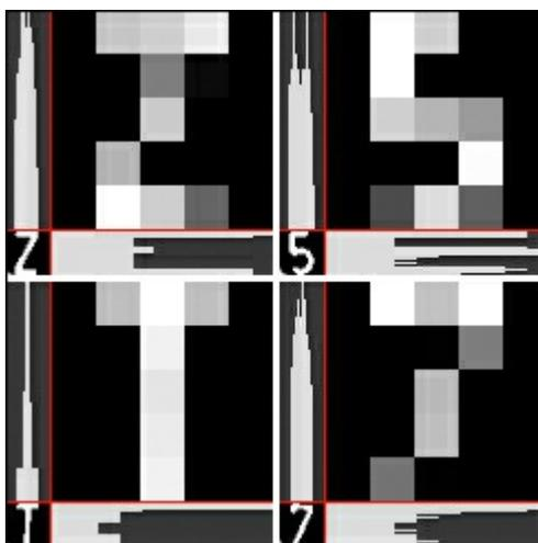
For each character, we count the number of pixels in a row or column with a non-zero value using the `countNonZero` function and store it in a new data matrix called `mhist`. We normalize it by looking for the maximum value in the data matrix using the `minMaxLoc` function and divide all elements of `mhist`
