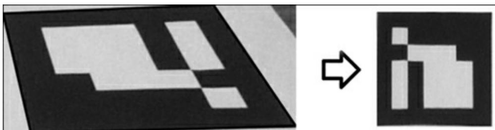
Now we can test the image to verify if it is a valid marker image. Then we try to extract the bit mask with the marker code. As we expect our marker to contain only black and white colors, we can perform Otsu thresholding to remove gray pixels and leave only black and white pixels:
