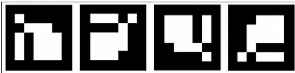
As there are four possible orientations of the marker picture, we have to find the correct marker position. Remember, we introduced three parity bits for each two bits of information. With their help we can find the hamming distance for each possible marker orientation. The correct marker position will have zero hamming distance error, while the other rotations won't.
