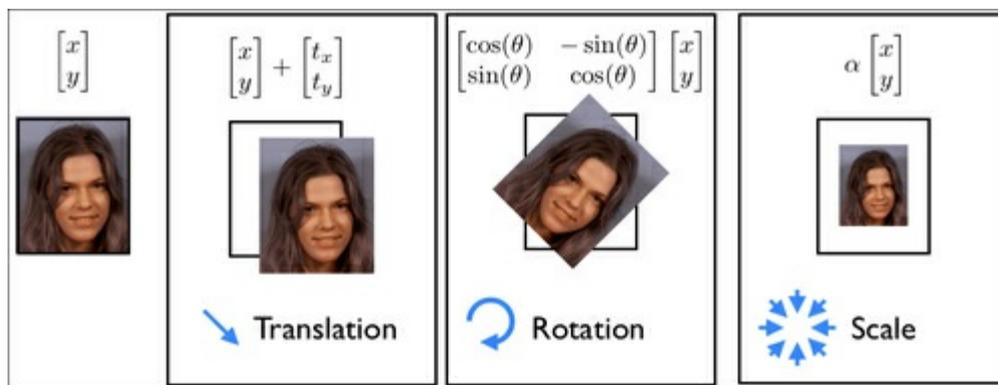
Mathematically, the objective of Procrustes analysis is to simultaneously find a canonical shape and similarity transform each data instance that brings them into alignment with the canonical shape. Here, alignment is measured as the least-squares distance between each transformed shape with the canonical shape. An iterative procedure for fulfilling this objective is implemented in the `shape_model` class as follows:
