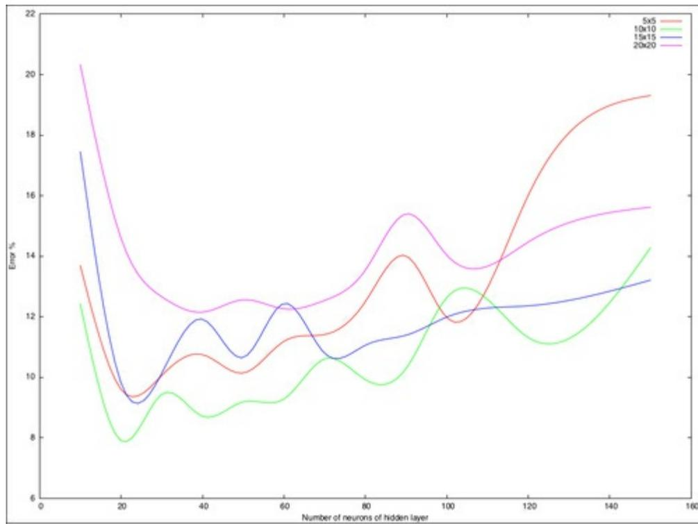
We can see that the lowest error is under 8 percent and is using 20 neurons in a hidden layer and characters' features extracted from a downsampled 10 x 10 image patch.
