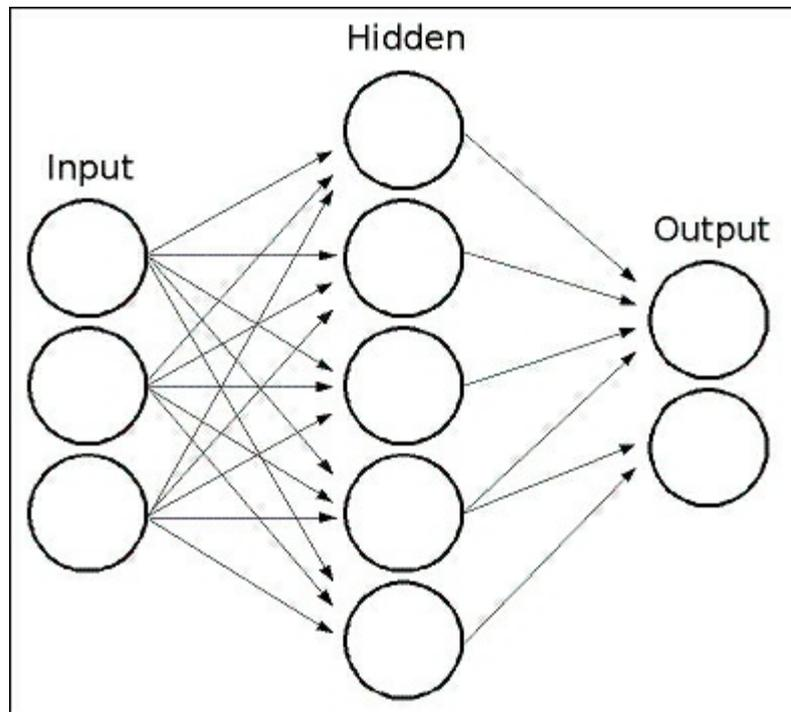
All neurons in an MLP are similar and each one has several inputs (the previous linked neurons) and several output links with the same value (the next linked neurons). Each neuron calculates the output value as a sum of the weighted inputs plus a bias term and is transformed by a selected activation function:
