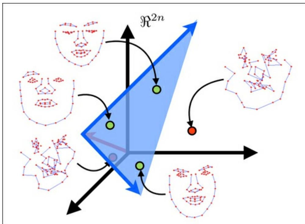
The procedure for finding the best low-dimensional subspace that spans a dataset is called Principal Component Analysis (PCA). OpenCV implements a class for computing PCA, however, it requires the number of preserved subspace dimensions to be prespecified. As this is often difficult to determine a priori, a common heuristic is to choose it based on the fraction of the total amount of variation it accounts for. In the `shape_model::train` function, PCA is implemented as follows:
