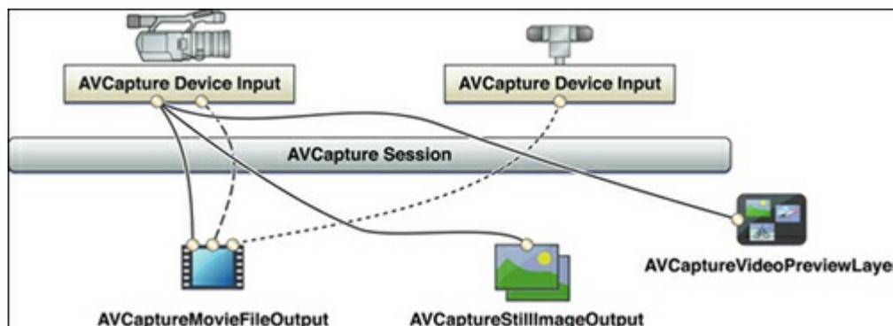
[AVCaptureSession](#) is a root capture object that we should create. Capture session requires two components—an input and an output. The input device can either be a physical device (camera) or a video file (not shown in diagram). In our case it's a built-in camera (front or back). The output device can be presented by one of the following interfaces:
