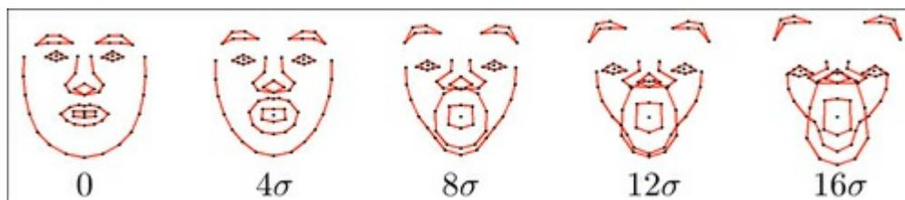
A simple way to prevent such deformation is to clamp the subspace coordinate values to lie within a permissible region as determined from the dataset. A common choice for this is a box constraint within  $\pm 3$  standard deviations of the data, which accounts for 99.7 percent of variation in the data. These clamping values are computed in the `shape_model::train` function after the subspace is found, as
