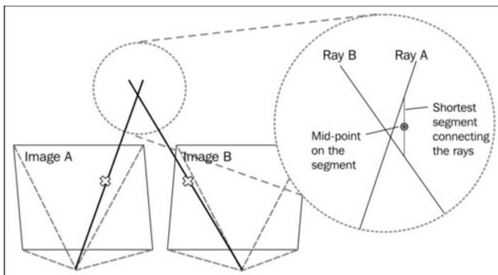
In reality, ray intersection is highly unreliable; H and Z recommend against it. This is because the rays usually do not intersect, making us fall back to using the middle point on the shortest segment connecting the two rays. Instead, H and Z suggest a number of ways to triangulate 3D points, of which we will discuss a couple of them in the Reconstructing the scene section. The current version of OpenCV does not contain a simple API for triangulation, so this part we will code on our own.
