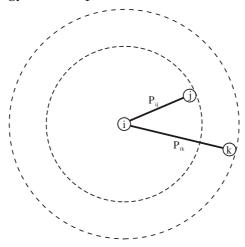
**Fig. 1:** The "wireless multicast advantage":  $P_{i,(j,k)} = \max\{P_{ij}, P_{ik}\}$
