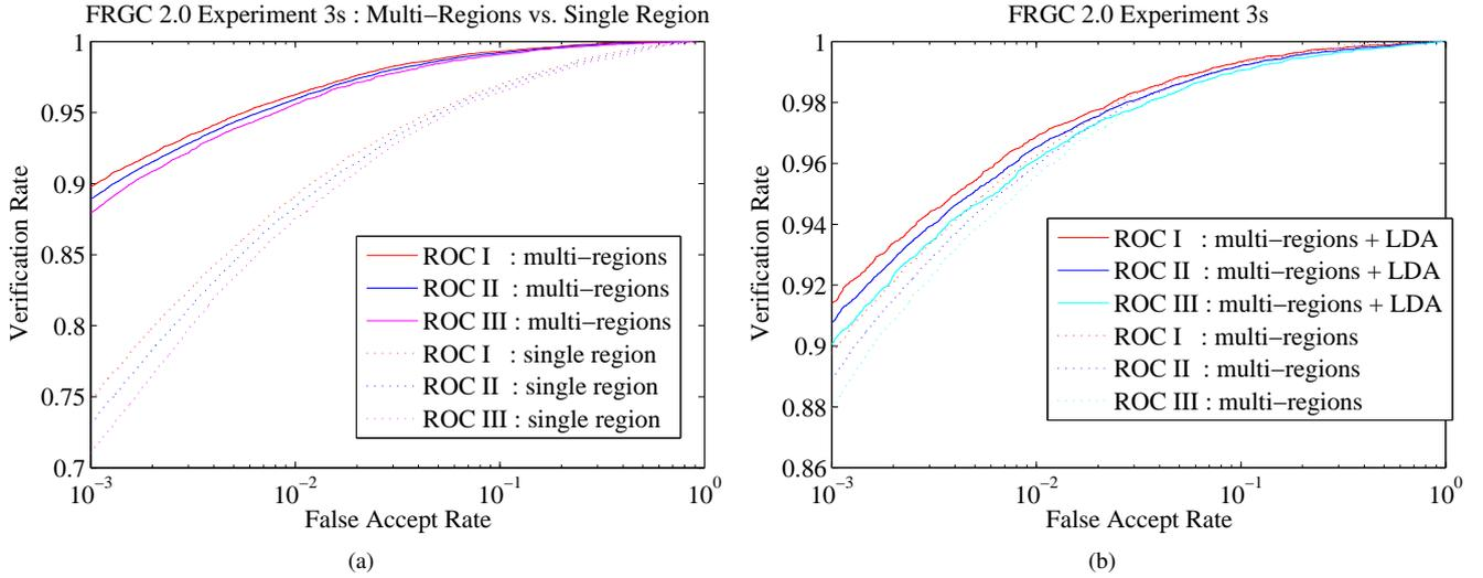
**Fig. 3.** ROC performance obtained by information fusion. (a) Fusion by sum rule (solid lines) and single region method (dashed lines). (b) Fusion by LDA (solid lines) and sum rule (dashed lines).
