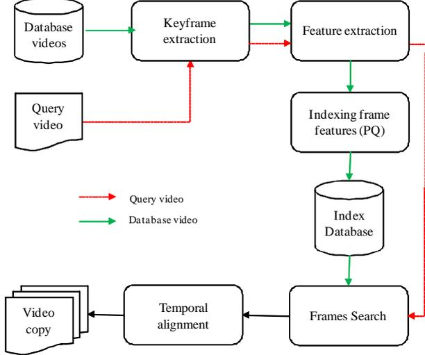
Figure 4. The proposed framework for video copy detection.
