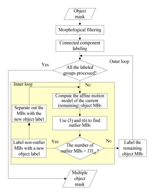
Fig. 4. Flowchart of the proposed object clustering scheme.
