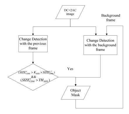
Fig. 3. Block diagram of object segmentation mask refinement.
