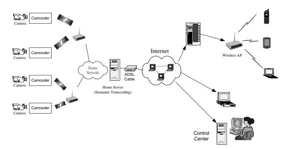
Fig. 1. Conceptual diagram of proposed intelligent networked home surveillance.
