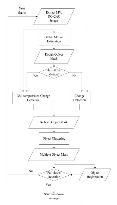
Fig. 2. Flowchart of the proposed compressed-domain fall incident detection scheme.
