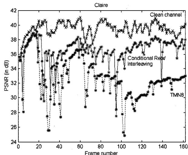
Fig. 7. PSNR comparison for the “Claire” sequence between TMN-8 in clean channel (-x-line), TMN-8 with packet loss and concealment (dashed -\*line), and our proposed conditional retransmission and interleaving scheme (solid -\*line). TMN-8 results in 12 frames skipped, while our proposed scheme has no frames skipped.
