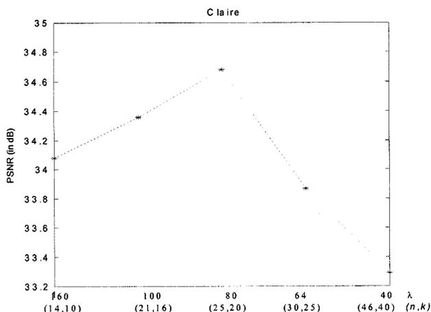
Fig. 4. Effects of different interleaving degree ( $\lambda$ ) and BCH code ( $n, k$ ) on video quality. Test sequence is "Claire."
