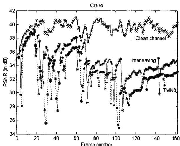
Fig. 5. PSNR comparison for the “Claire” sequence between TMN-8 in clean channel (-x-line), TMN-8 with packet loss and concealment (dashed -\*line), and our proposed interleaving scheme (solid -\*line). TMN-8 results in 12 frames skipped, while our proposed scheme has no frames skipped.
