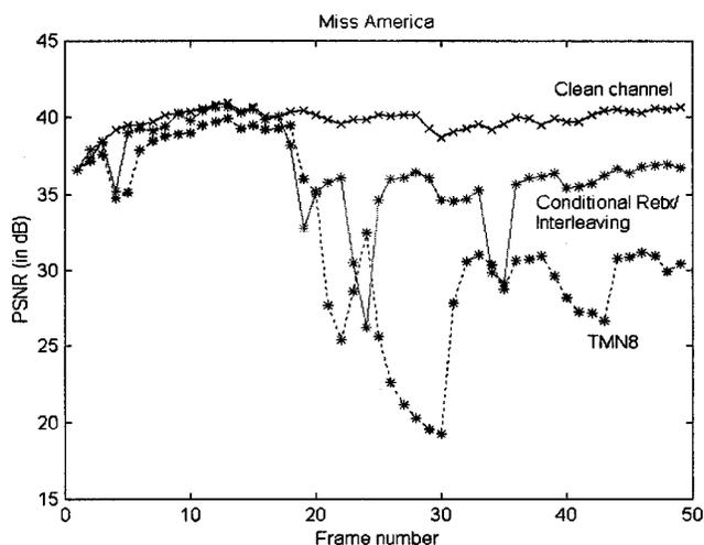
Fig. 8. PSNR comparison for the “Miss America” sequence between TMN-8 in clean channel (-x-line), TMN-8 with packet loss and concealment (dashed -\*line), and our proposed conditional retransmission and interleaving scheme (solid -\*line). TMN-8 results in 7 frames skipped, while our proposed scheme has no frames skipped.
