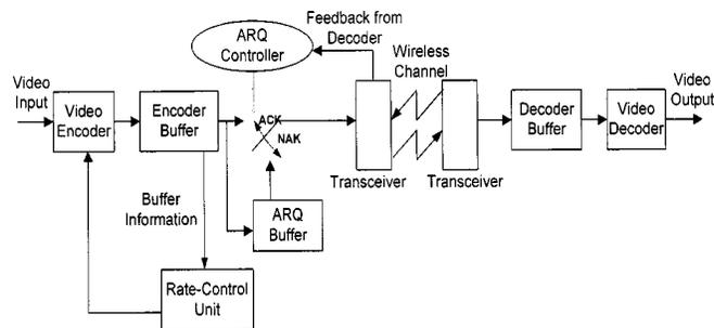
Fig. 1. Block diagram of a retransmission-based wireless video system.
