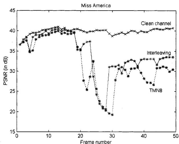
Fig. 6. PSNR comparison for the “Miss America” sequence between TMN-8 in clean channel (-x-line), TMN-8 with packet loss and concealment (dashed -\*line), and our proposed interleaving scheme (solid -\*line). TMN-8 results in 7 frames skipped, while our proposed scheme has no frames skipped.
