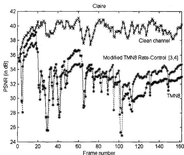
Fig. 2. PSNR comparison for the "Claire" sequence between TMN-8 in clean channel (-x-line), TMN-8 with packet loss and concealment (dashed -\*line), and the scheme proposed in [3] (solid -\*line). TMN-8 results in 12 frames skipped at the encoder while the proposed scheme in [3] has no frames skipped.
