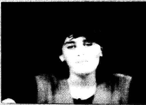
Figure 8. Miss America sequence simulation result. Frame number: 115, bit rate: 64 kbs, frame rate: 10 frames/s, S/N (luminance): 37.7 dB.
